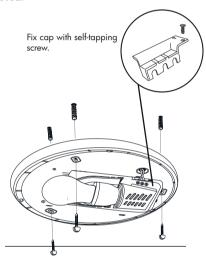
Open the lamp by lightly turning the glass anti-clockwise. Lead the mains cable on the back of the lamp through the rubber bushing. Mark drill holes on the ceiling or wall. Drill suitable holes and push the plugs tightly into the holes. Screw on the lamp.
