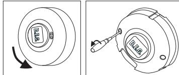
The circular cover ring must be removed prior to assembly. To do this, twist the lens anticlockwise through approximately 5° and lift off.
